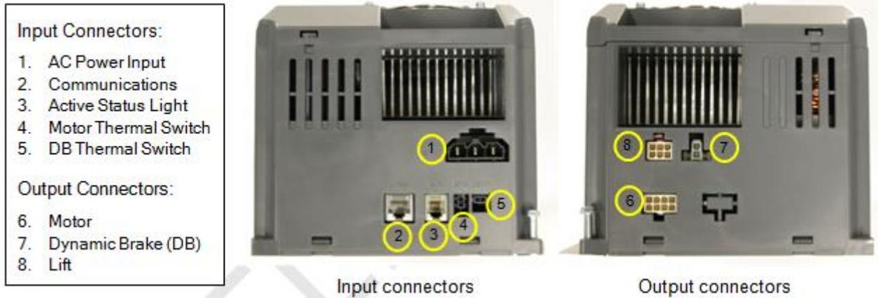
Figure 15: Motor Controller Connector Pin 1 location
